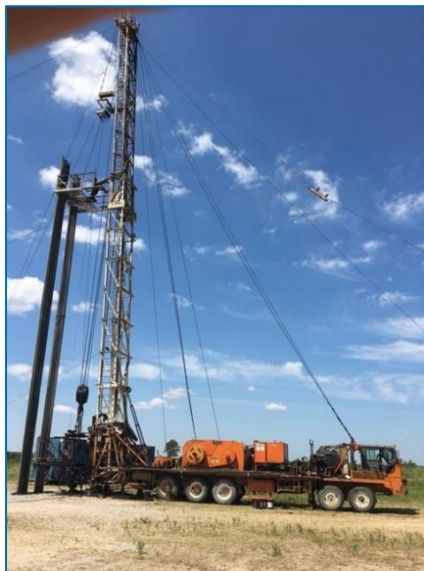
Figure 1. Workover Rig on location, Mitchell 1-12 well, Carter County
